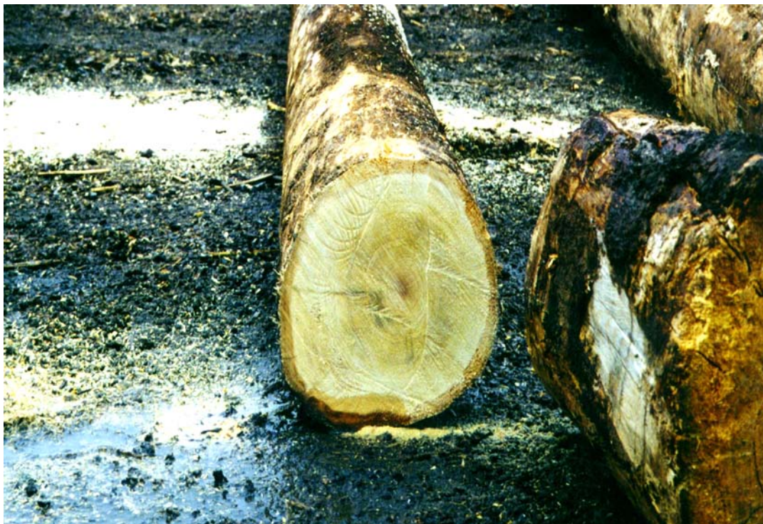
Figure 6.1 Sap rot encompassing 100% circumference of the outside collar
