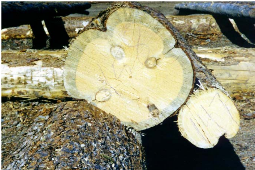
Figure 6.3 Example of a log with blue stain which should not be confused with sap rot
