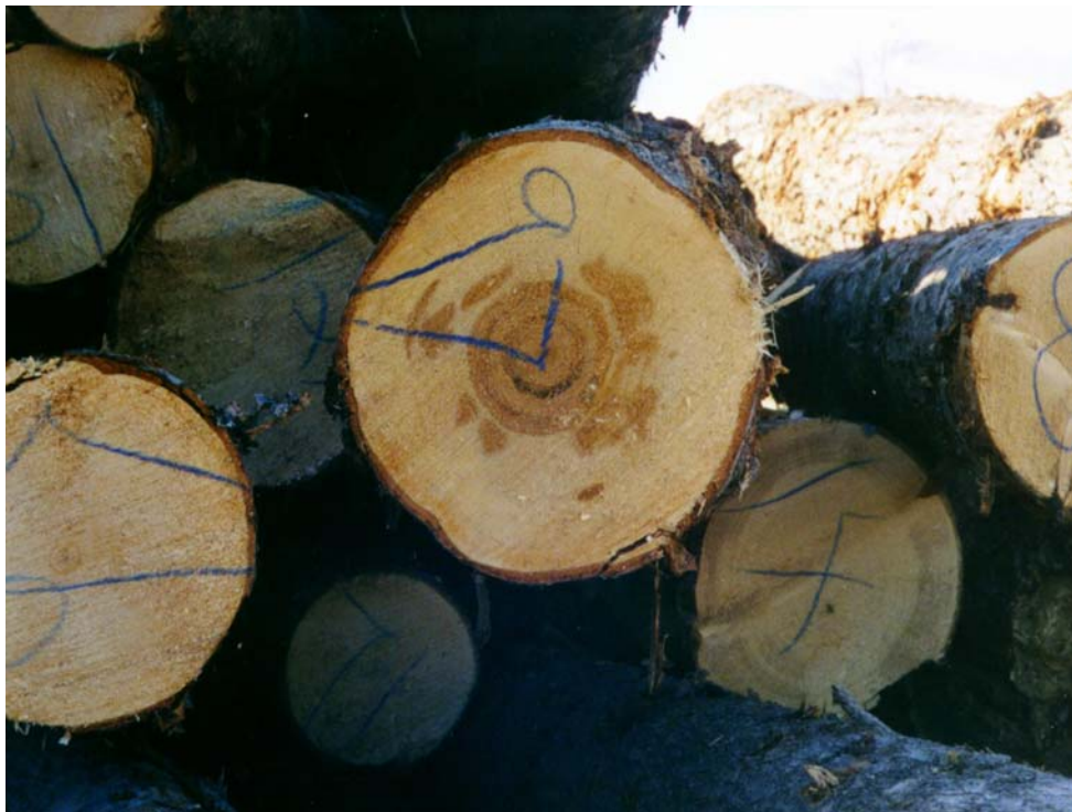
Figure 7.3 Heart rot with scattered areas of pocket rot
