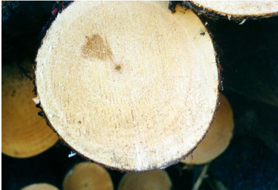
Figure 8.7 Triangular rot in different sizes
