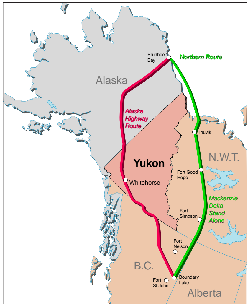
Route showing the northern gas pipeline options.
