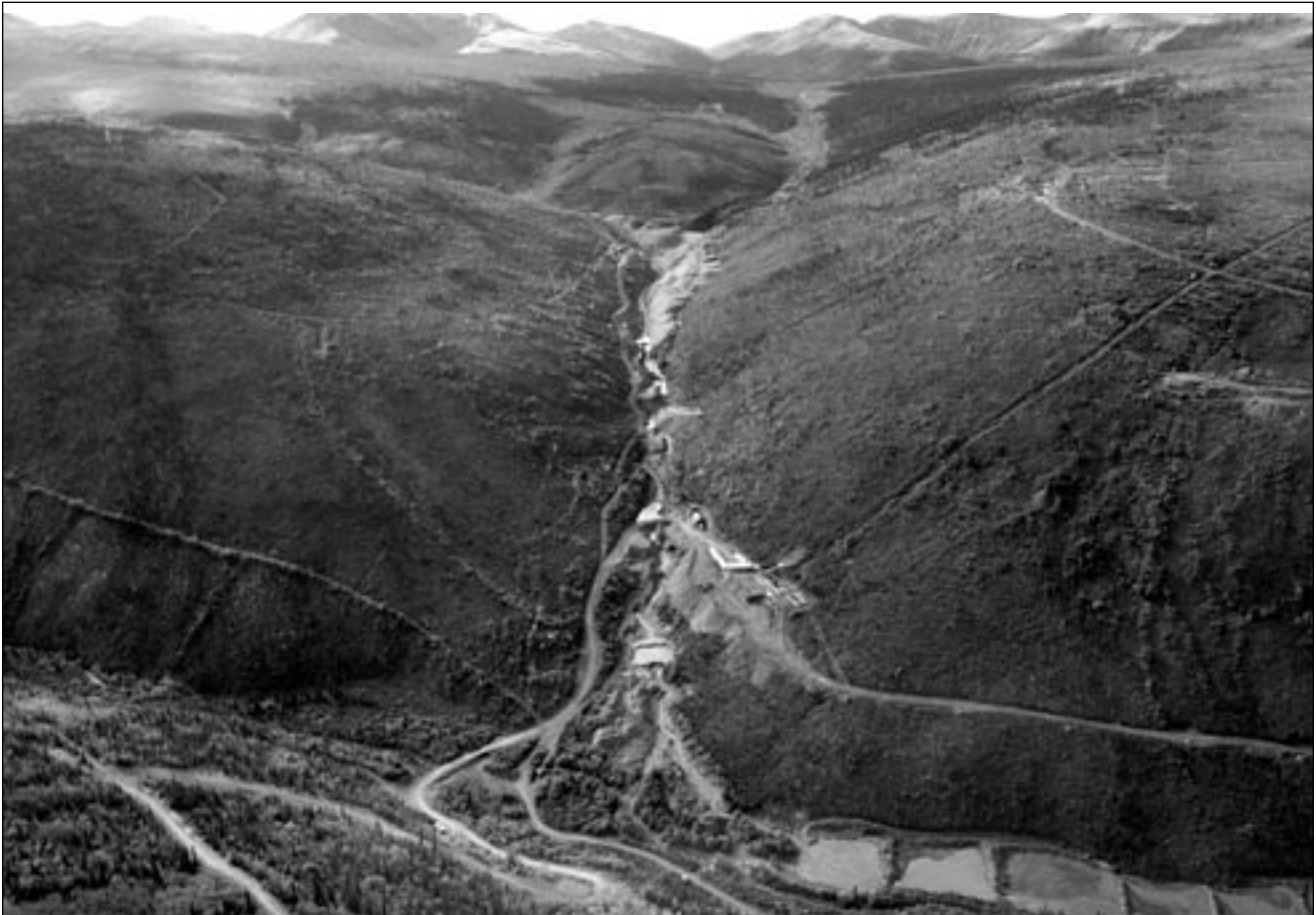
WATER is usually used as the transporting or washing agent to remove the gold from the sand and gravel. The water is often pumped from a stream into an elaborate system of pumps and settling ponds. Later it is returned to the stream once the fine sediments have settled.
