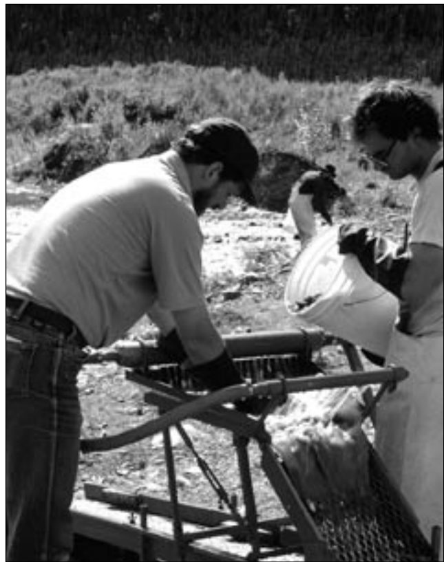
Working the sluicebox, an essential part of the processing of placer gravel.
