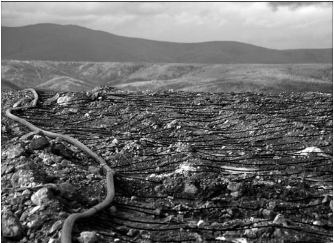
Drip lines were part of the leach pad at the Brewery Creek Mine, 1997.
