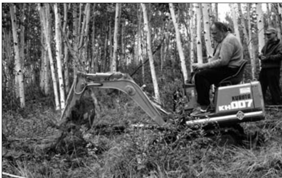
Whenever possible, smaller and lighter excavators are used to sample a placer deposit.
