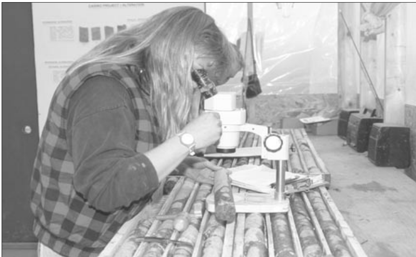
A geologist examines core samples, a critical step in exploration.
