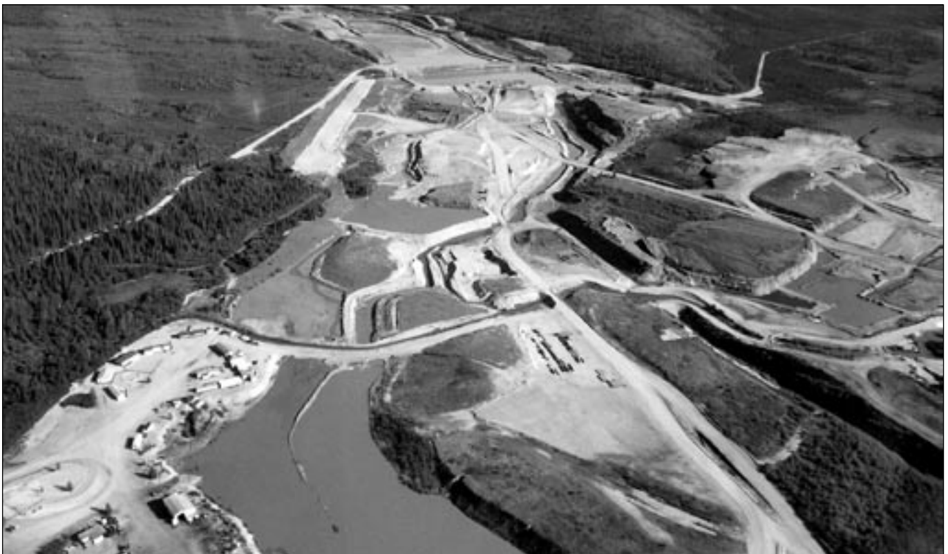
Placer operation in the Klondike area. Settling ponds are visible in the foreground. Dark grassy areas were worked the previous year and are quickly revegetating.
