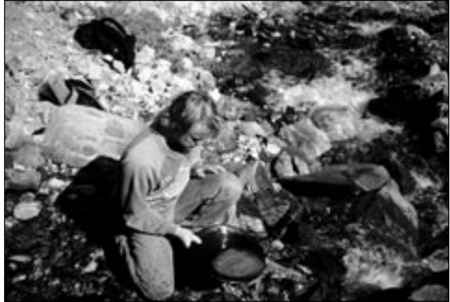
The GOLD PAN is used to test prospective gravels for gold.
