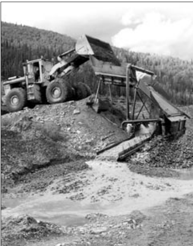
Gold-rich gravel is dumped into a sorting box. Larger rocks come out in a pile and the finer particles run through a sluicebox.
