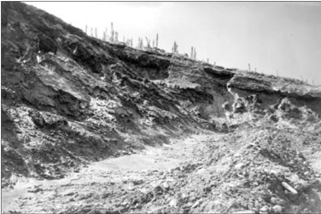
Placer mining in the Sixtymile area; stripping in ice-rich permafrost soils, April, 1996.
