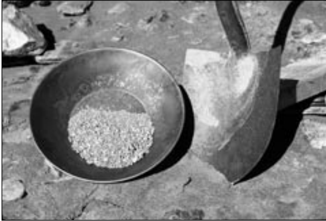
The GOLD PAN is used to test prospective gravels for gold.
