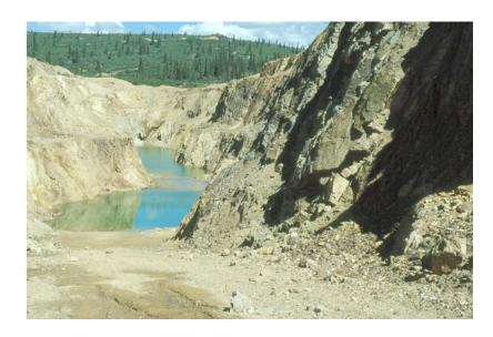
c) The Pit: the main pit collects water and must be pumped out to prevent water from flowing through an old underground tunnel and into Pony Creek. The water is pumped out and treated as it contains small amounts of zinc. This treated water is released into Dome Creek. The water coming into the pit is partially evaporated during the summer. Although the water level does rise in the summer it gets lower over the winter.
