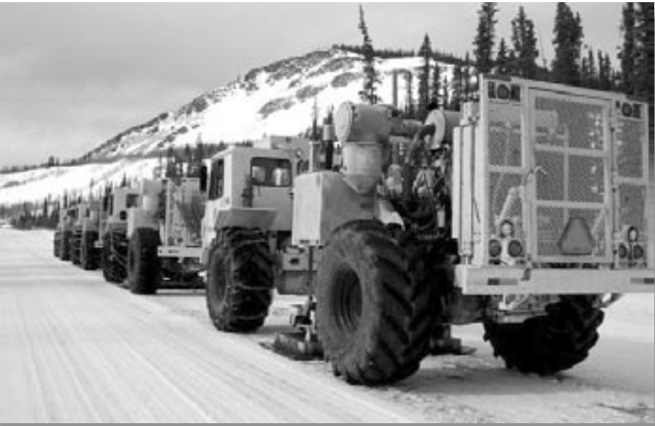
Vibreosis trucks conduct seismic work near Carmacks, Yukon as part of the Yukon Geological Survey's resource assessment work in the Whitehorse Trough basin.
