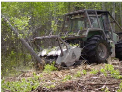
Mulcher selectively removing trees
