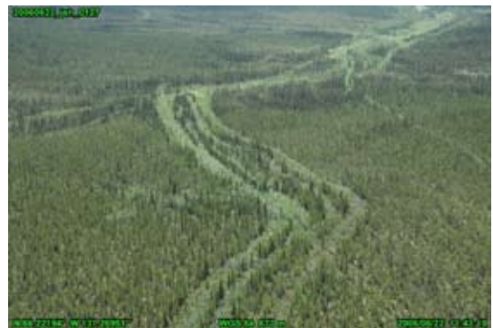
Parallel lines created on a travel route. Cause likely poor consideration of ground conditions or seasonal timing Eagle Plains area north of the Dempster highway
