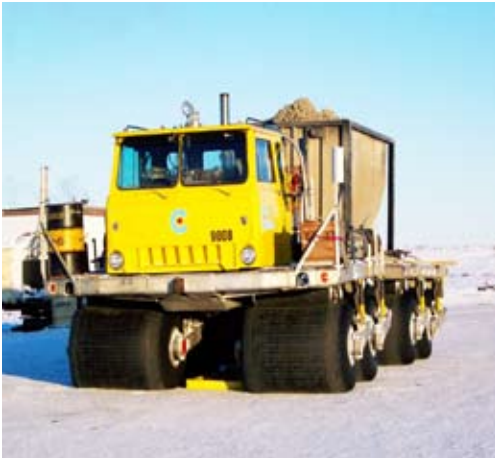
CATCO low ground pressure vehicle during ConocoPhillips Canada, Mackenzie Delta low ground pressure vehicle trial. Photo ConocoPhillips Canada
