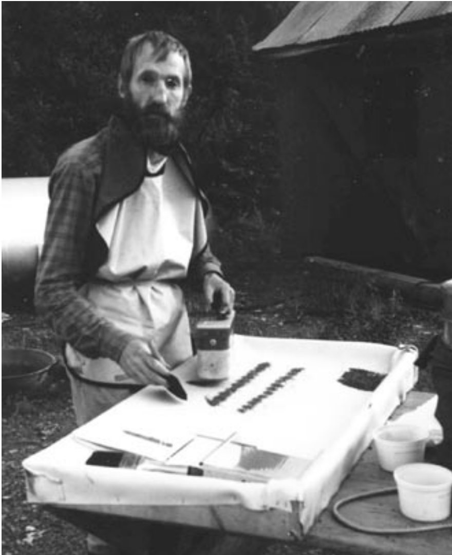
Yukon mining engineer Randy Clarkson uses radio tracer technology to test the efficiency of gold recovery. — Randy Clarkson photo
