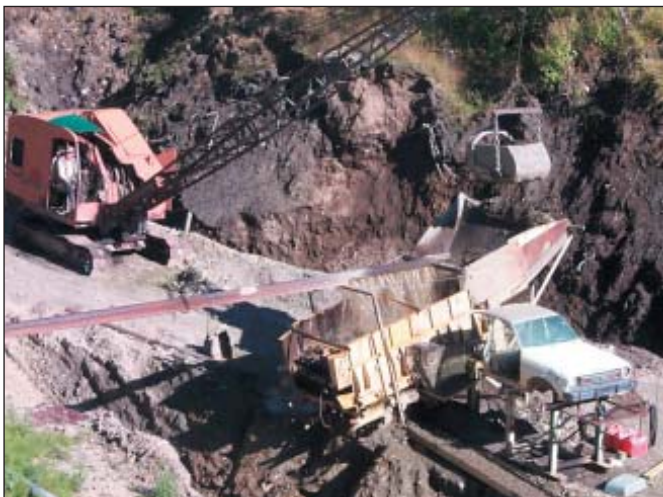
Close-up view of Alf Roberts using a drag line with ½ yard bucket, to dig pay gravel and feed the wash plant, in Homestake Gulch.
