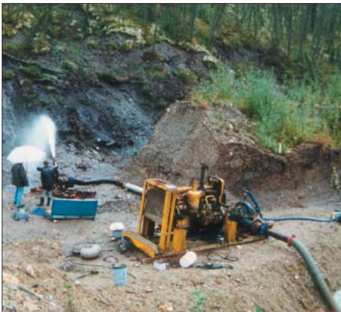
John Erickson on Hunker Creek. Monitor being used to thaw black muck to expose side pay.
