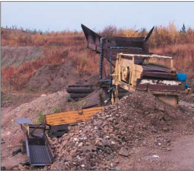
Close up view of the dump box, shaker plant and sluice runs used by Everett Kissler on 7 Pup, a left limit tributary to Victoria Gulch on Upper Bonanza Creek.
