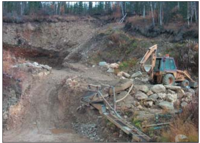
Looking at the mining cut on the left limit of upper Gauvin Gulch where W.L. Roberts used this small back hoe/loader to feed the wash plant in the foreground. Several large boulders removed from the pay zone can be seen near the wash plant.
