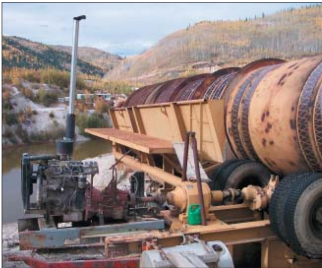
Large trommel and dump box used by Clive Nicholson, set up among White Channel gravel tailings, near Lovett Gulch on Bonanza Creek.
