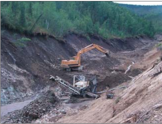
Looking upstream on O'Neil Gulch at Henry Gulch Placers using an excavator to dig pay gravel and feed the wash plant.
