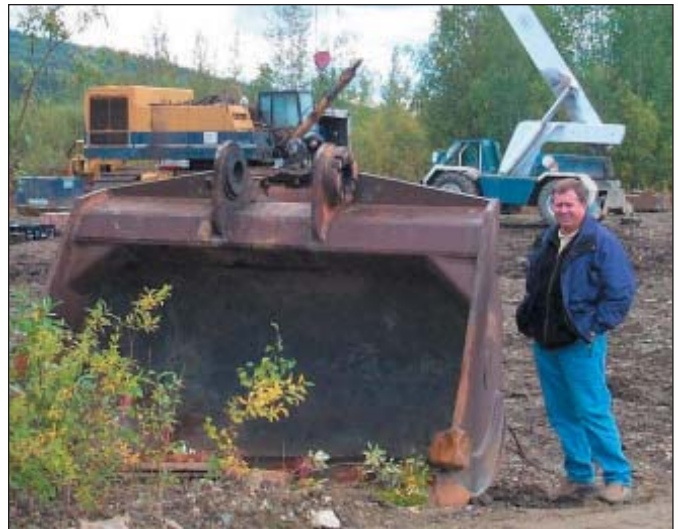
Al Rothwell stands beside a PC1000 Komatsu 6 cubic yard bucket.
