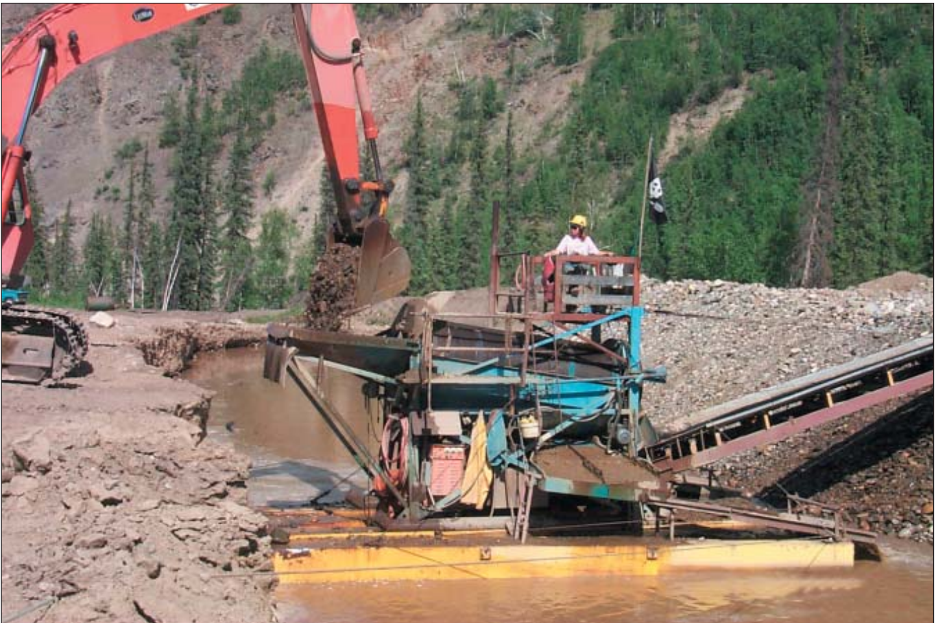
Leslie Chapman atop of Fortymile Placers' floating trommel while Bill Claxton feeds pay material.
