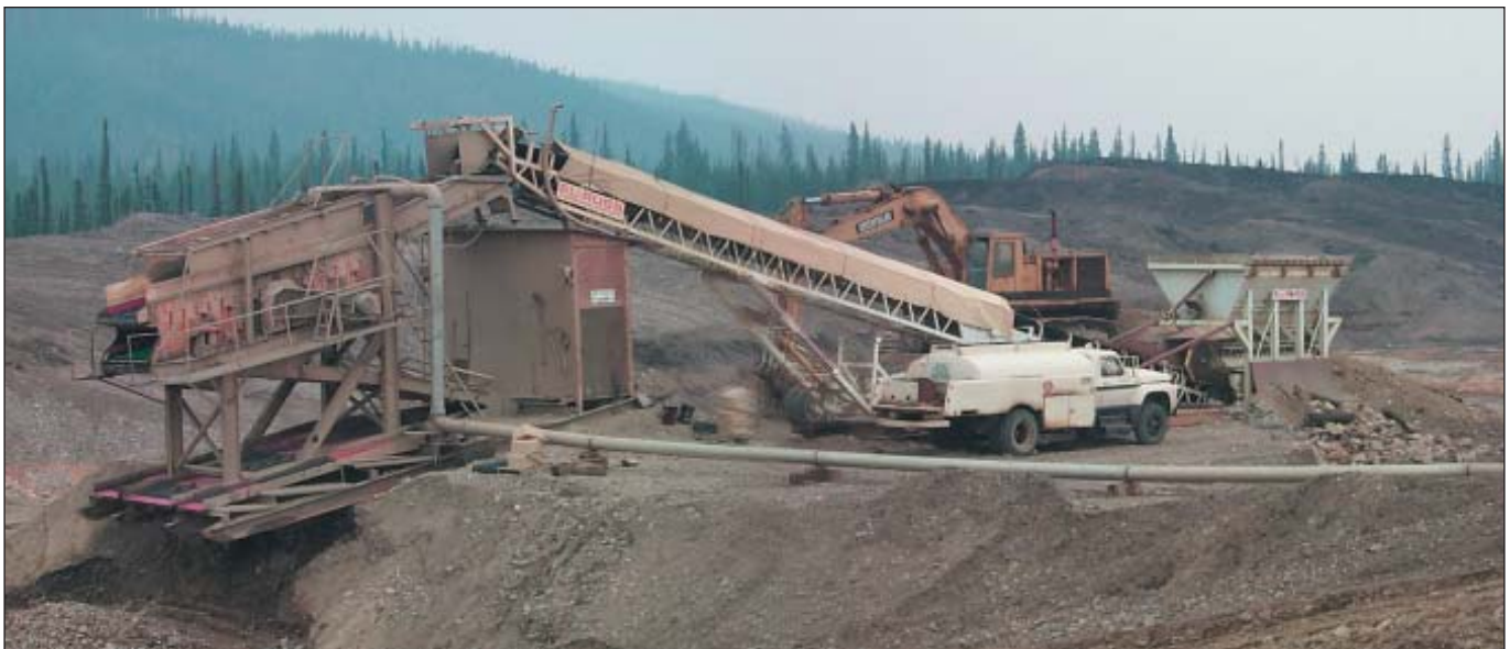
Eldorado Placer's sluice plant operating in the Sixtymile River area downstream from 5 Mile Creek in 2002.
