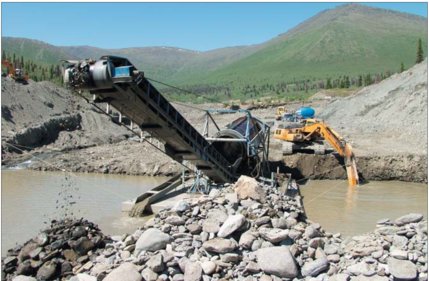
Soda Computing's New Zealand-style floating wash plant at Fourth of July Creek.
