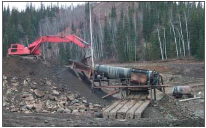
The trommel used by Favron Enterprises for their operation on Last Chance Creek in 2002.
