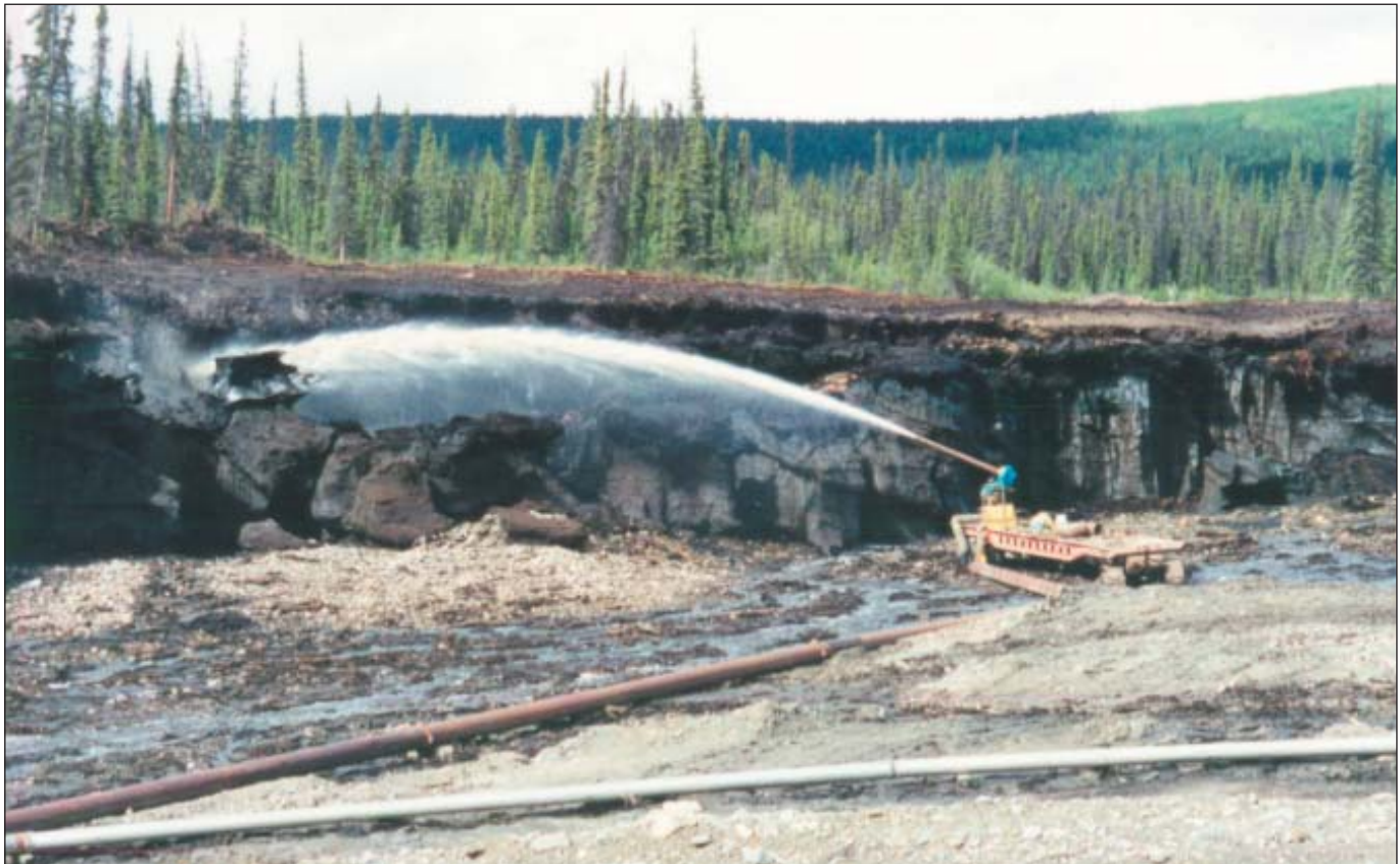
The automated hydraulic monitor used at Laskey Pup on Gold Run Creek by Ray Lizotte and Brent Construction.
