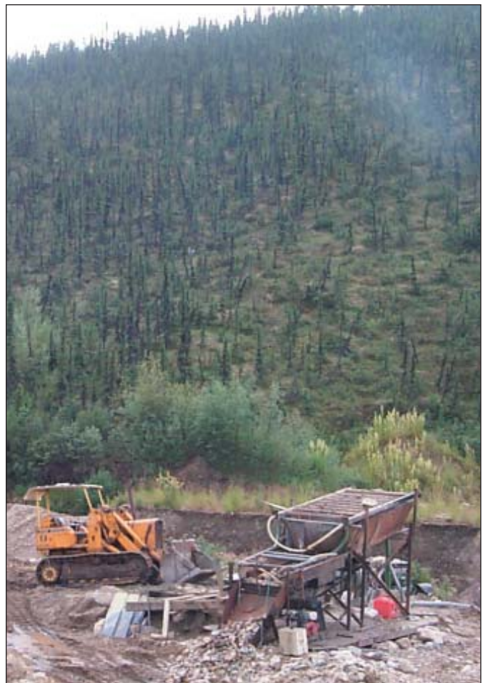
Small track-loader and wash plant used by Chesla McGee on Upper Bonanza Creek.
