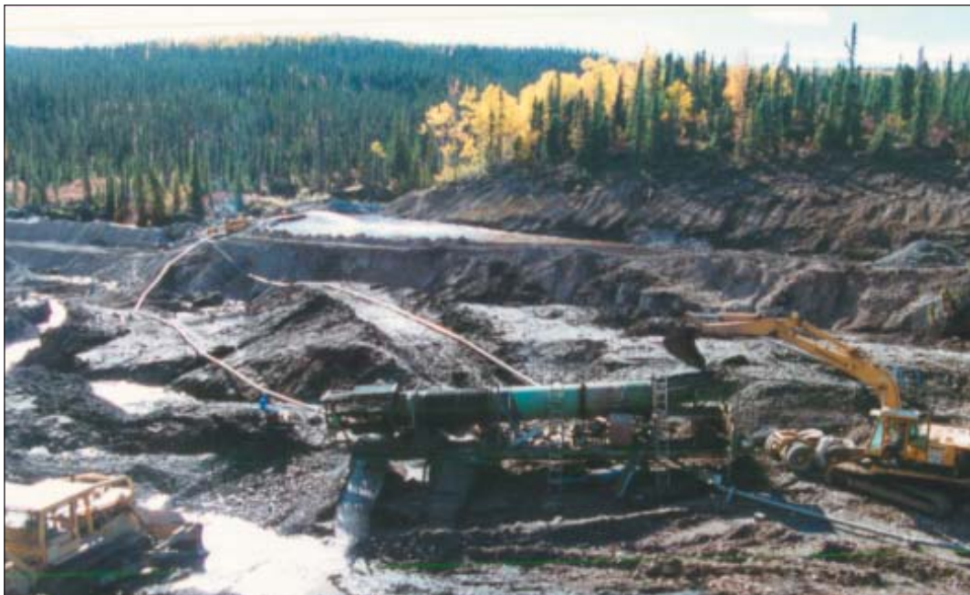
Excavator feeding pay material to Rod Smith's 4-foot by 32-inch trommel on Blackhills Creek.
