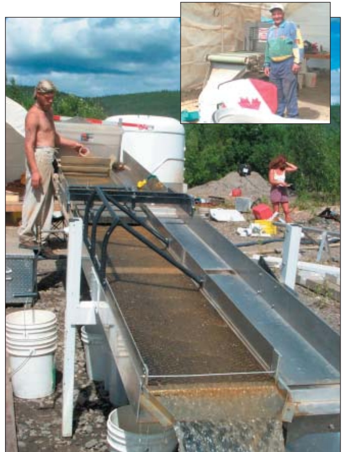
ISSL sluice runs on Indian River. (inset) Pete Risby stands beside rare earth magnet conveyor.
