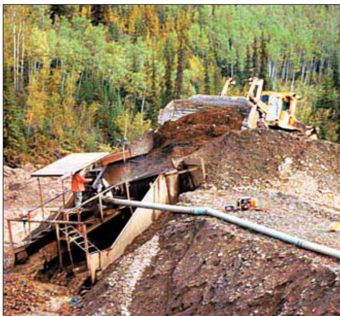
Midas Rex sluicing operation on Indian River.
