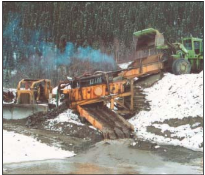
David Laurenson, Childs Gulch. Note the bulldozer pushing aside oversized tailings.
