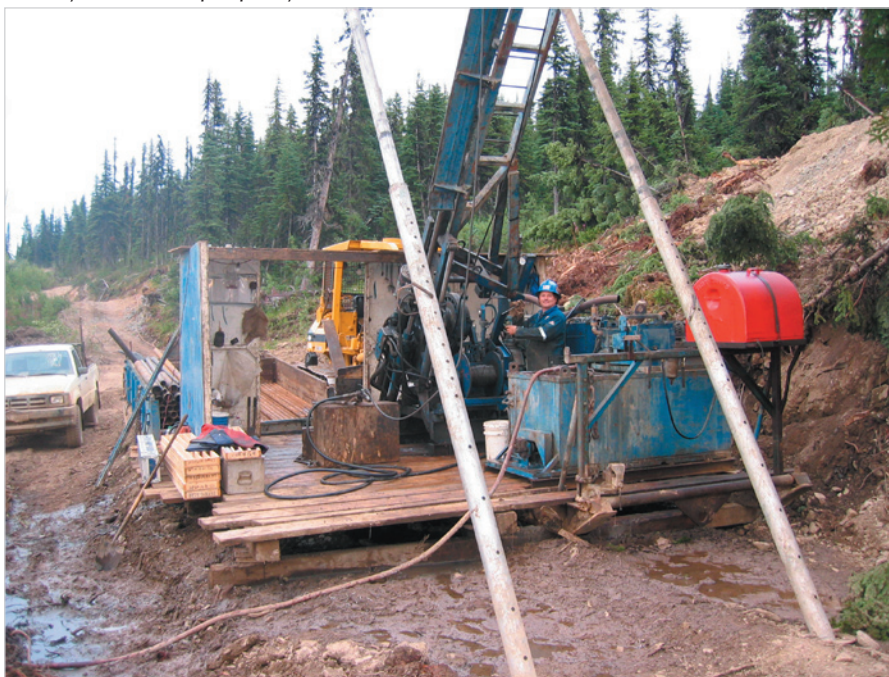
Figure 13. Diamond drilling on the Hyland Gold property.
