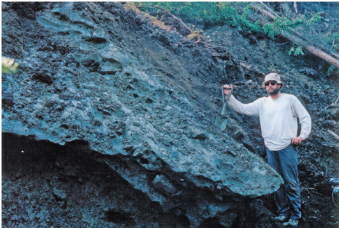
Figure 9. Massive ice in the old colluvial unit, YT slide.
