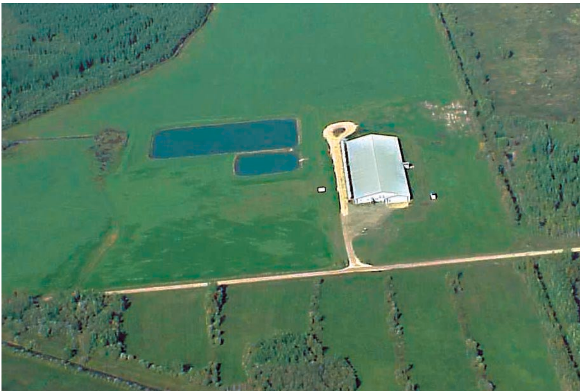
Earthen storage structure for liquid manure.
