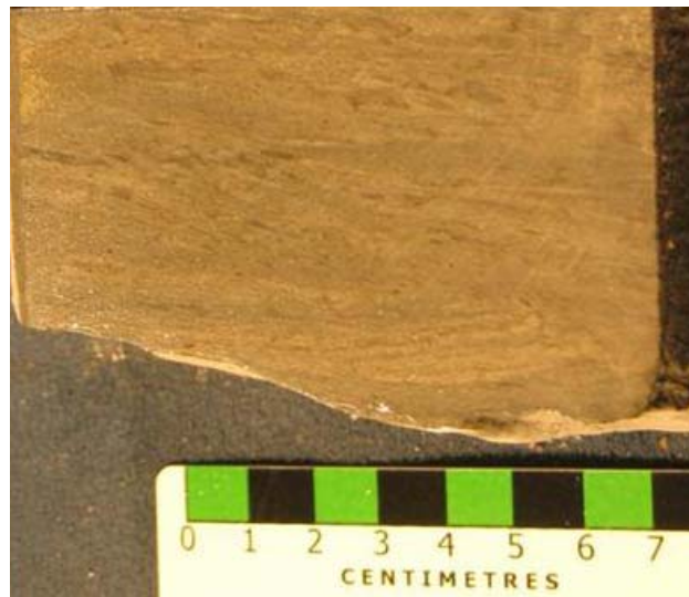
Figure 8 – Middle Bakken Member Crossbedding. Lithofacies 1. This core photo was taken at a drilled depth of 1080.6 m. Taken of 10-31-7-29 WPM.
