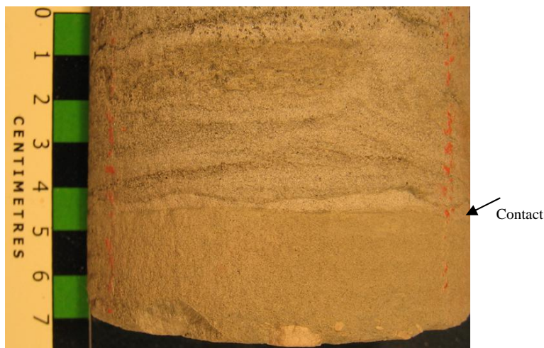
Figure 6 – Three Forks Formation Top. A sharp contact between the Three Forks and Middle Bakken. A rare occurrence. Photo taken at a drilled depth of 1082.7 m from core of a well located at 4-6-7-29 WPM.
