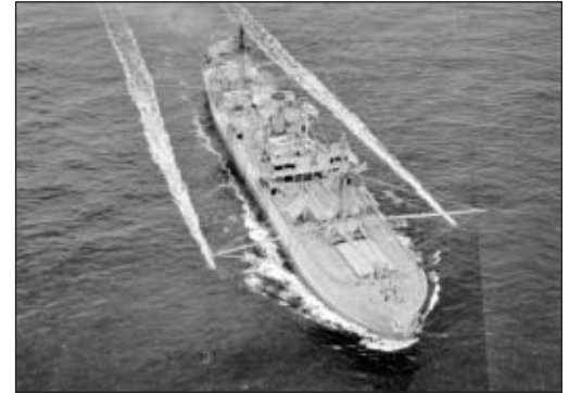
MERCHANT SHIP FITTED WITH ANTI-TORPEDO NETS, NEAR SYDNEY, N.S. (NAC PA152034)
