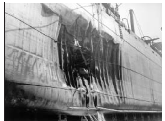
TORPEDO EXPLOSION DAMAGE TO THE HULL OF SS FORT CAMOSUN . (NAC PA190186)
