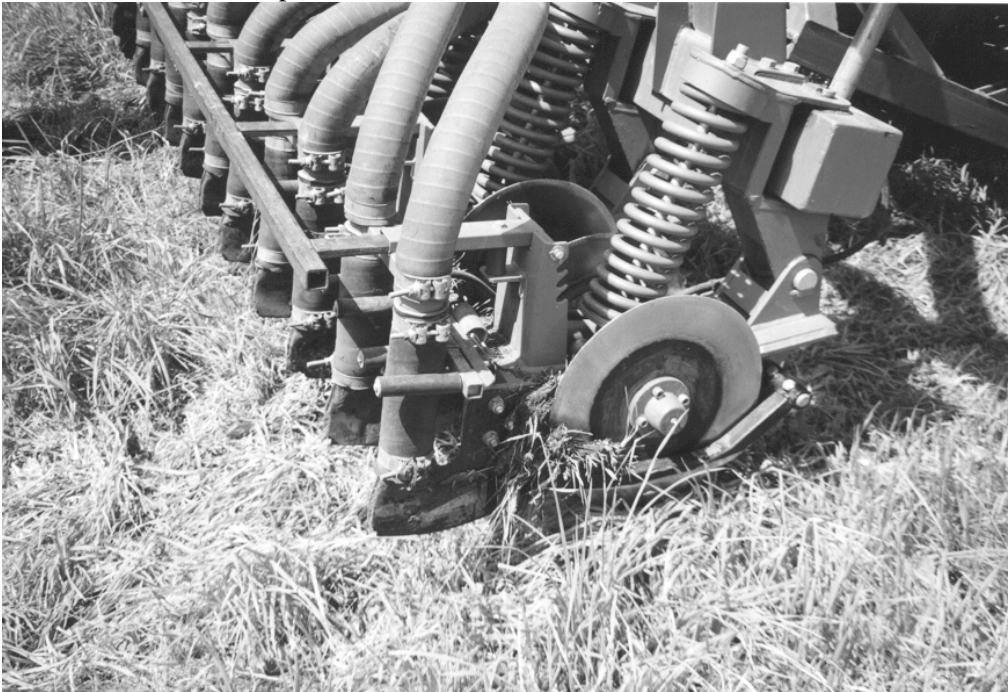
Figure 3a. Greentrac injector (knife-type) used for injection treatment in forage fields.
