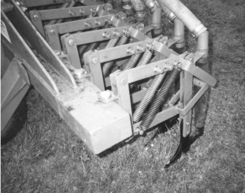
Figure 3b. Greentrac Sleighfoot used for sub-canopy application treatment in forage fields.
