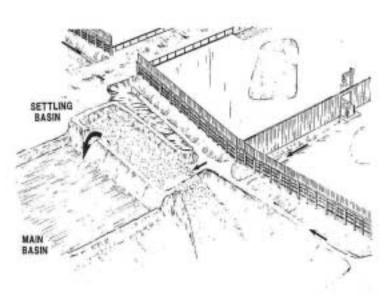
Larger facilities should consider using a two-stage collection basin. The first stage is a settling basin, which allows most of the solids in the runoff to be separated from the liquid. The settling basin should be relatively shallow, from 0.6 to 1.2 m (2 to 4 ft) deep. It should have an area of 2.5 percent of the total collection area. The second stage is then the main collection basin.
