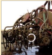
Fig. 1. Low disturbance Injection System
