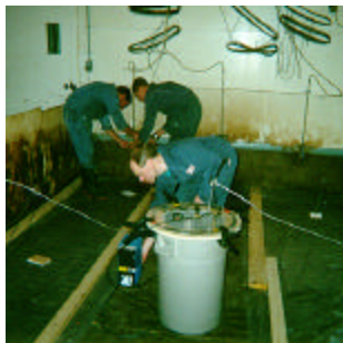
Air sampling set up during indoor trials
