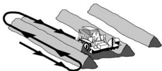
Figure 2a. Open windrows with mechanical turning. From Rynk, R. et al. 1992.
