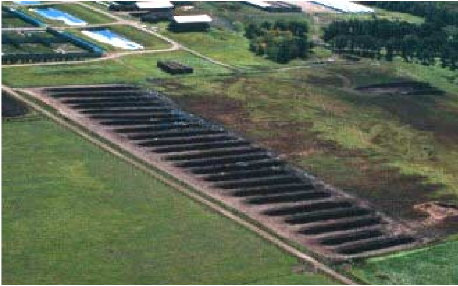
Figure 3. Photograph of the 5 acre composting site at Brandon Research Centre which can accommodate 8000 tonnes of raw manure for composting.
