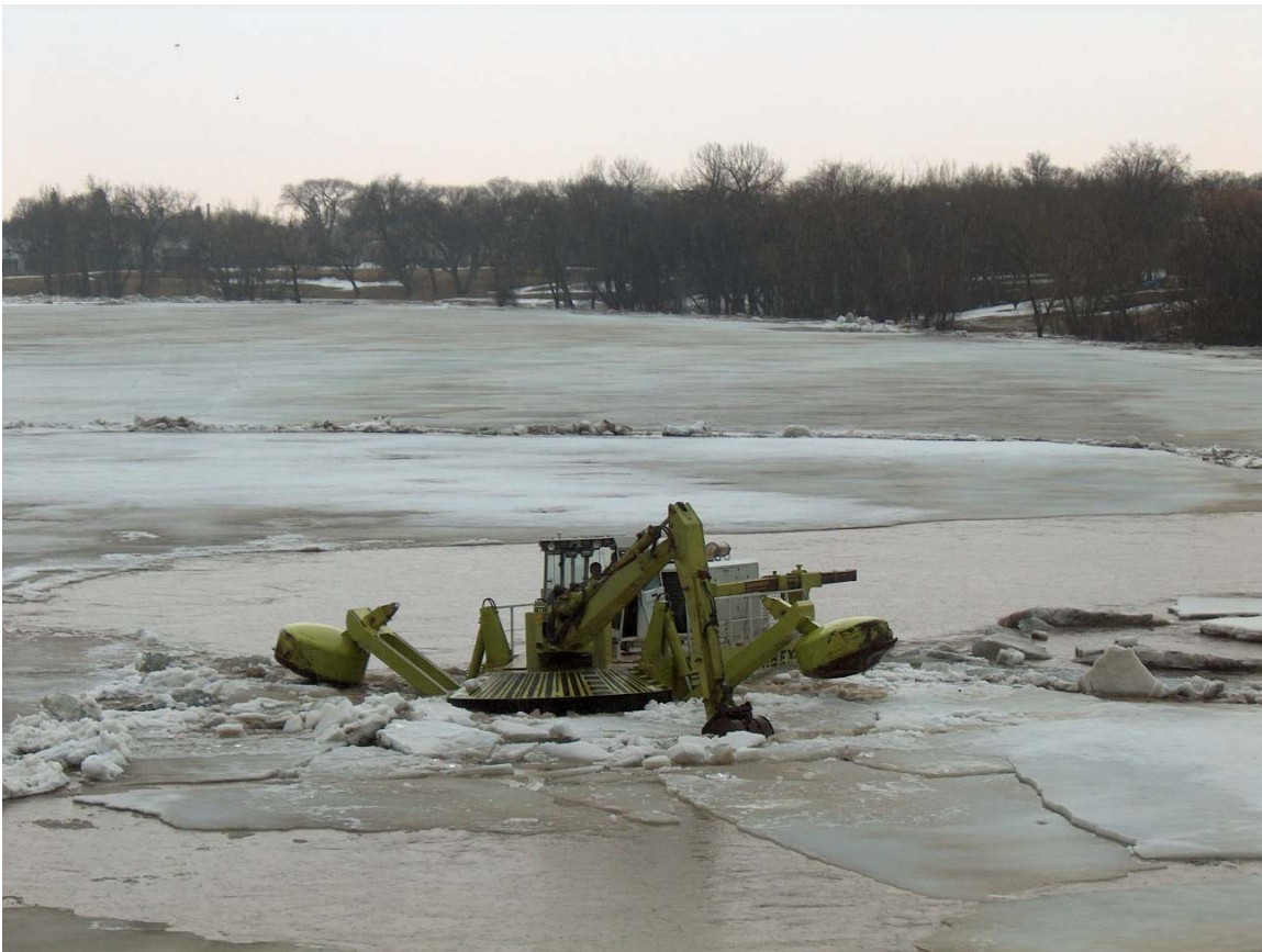
Figure 3 – Amphibex Ice Breaker at Redwood Bridge – April 4, 2005
