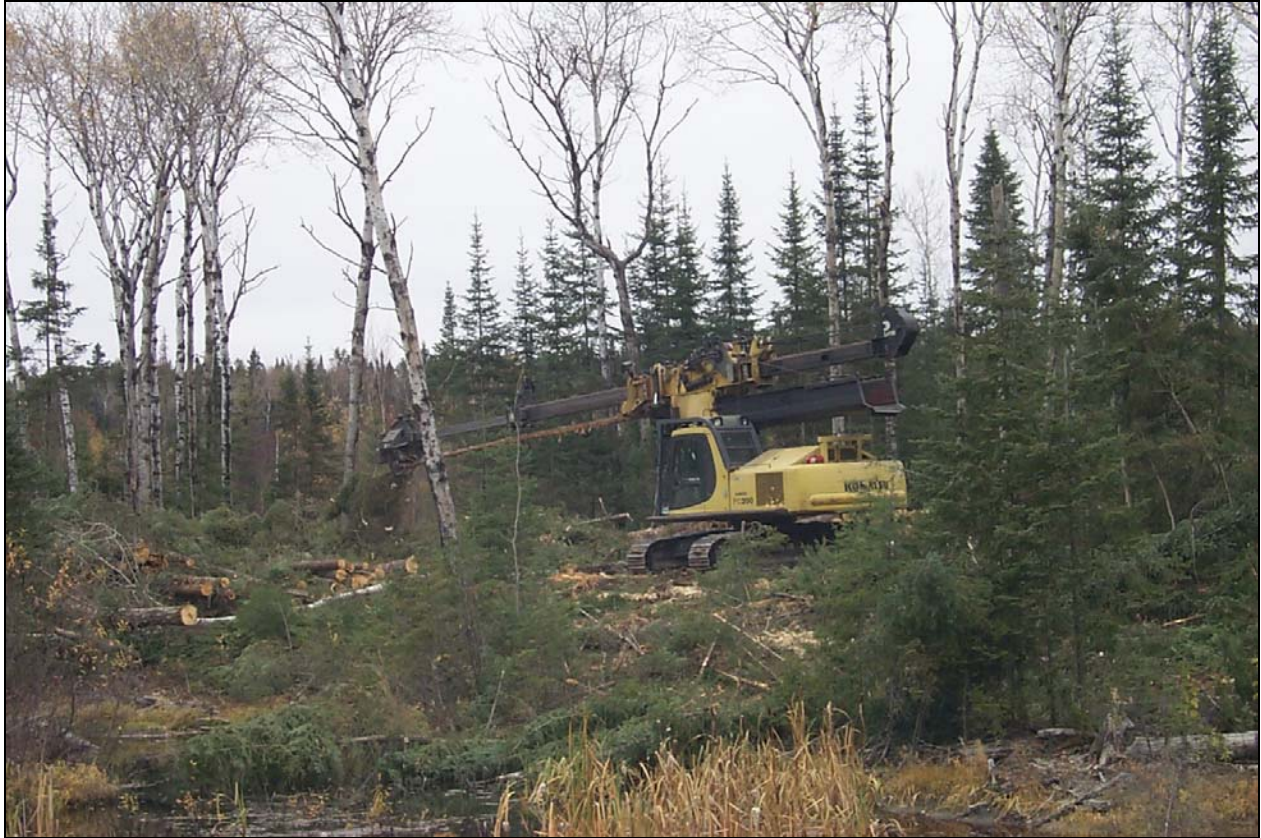
Figure 1. An example of in-block limbing.
