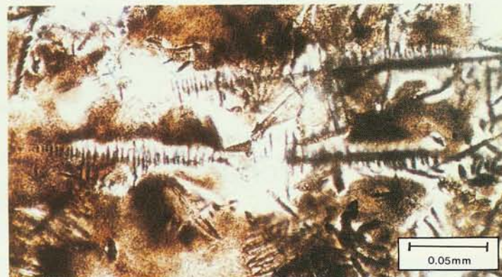
Figure 10 Glassy to partly devitrified fragments with skeletal crystals (bar scale in mm)
