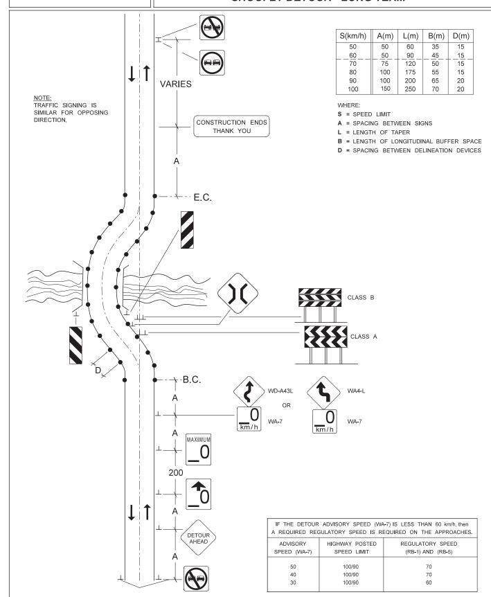
NOTE: IF A REGULATORY SPEED REDUCTION IS NOT REQUIRED, THEN MAINTAIN A DISTANCE OF 150m BETWEEN THE C-2 AND THE C-4.
