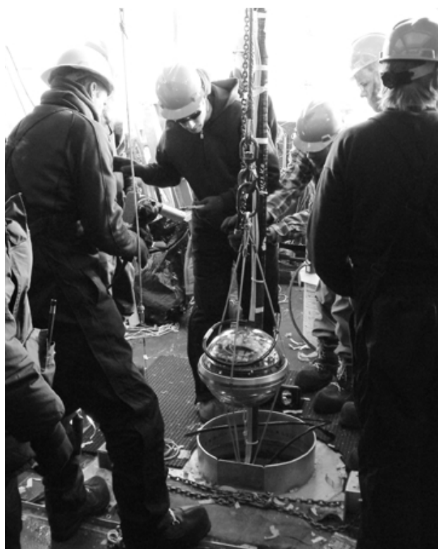
Figure 3 Ice Cube workers lowering detector string and module.
