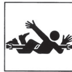
Figure 2.8.e. This sign warns of a potential PTO entanglement.
