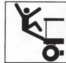
Figure 2.8.f. This safety sign warns of a potential fall hazard. Always use handholds. Falls account for a large number of agricultural injuries and fatalities each year.
