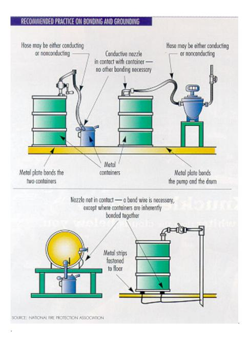
This kind of static situation can be controlled by reducing flow rates, avoiding violent splashing in the tank and allowing for "relaxation" time (simply waiting until the static charges dissipate) before gauging the tank
