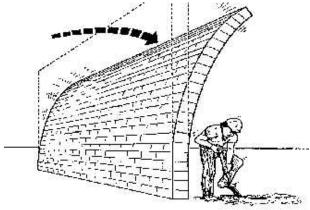
During construction, masonry walls lack the support provided by integral elements of the completed structure. When an unbraced or poorly braced masonry wall is blown over by the wind, It may result in extensive damage to property and equipment, serious injury or even loss of life. Temporary bracing must be installed to adequately support the wall until permanent structural members are in place.
