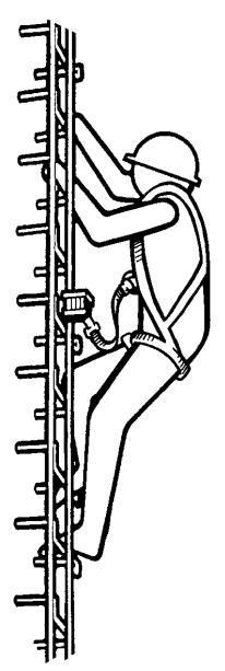
A worker fell to his death from a ladder attached to the outside of a metal grain bin. Fall protection equipment was not used on the six-meter high ladder.
