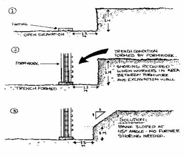
**BE AWARE**] An open excavation may become a trench excavation as the project proceeds. A concrete basement wall constructed in an open excavation 2.0 metres (6.6 feet) deep, now requires shoring or veeing out if workers are required to work on the outside wall between the concrete and earth.
