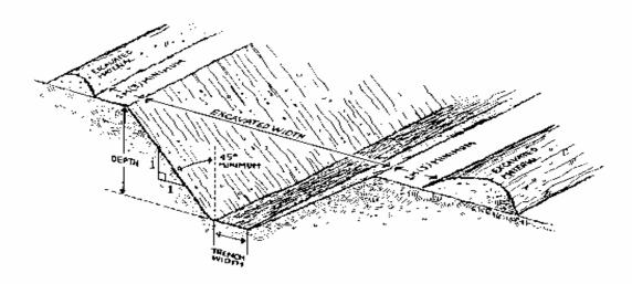
A combination 1:1 (45\*) slope and vertical face may be used, as long as the vertical face does not exceed 1 metre (3 feet) and the overall depth of the excavation is not greater than 5 metres (15 feet).
