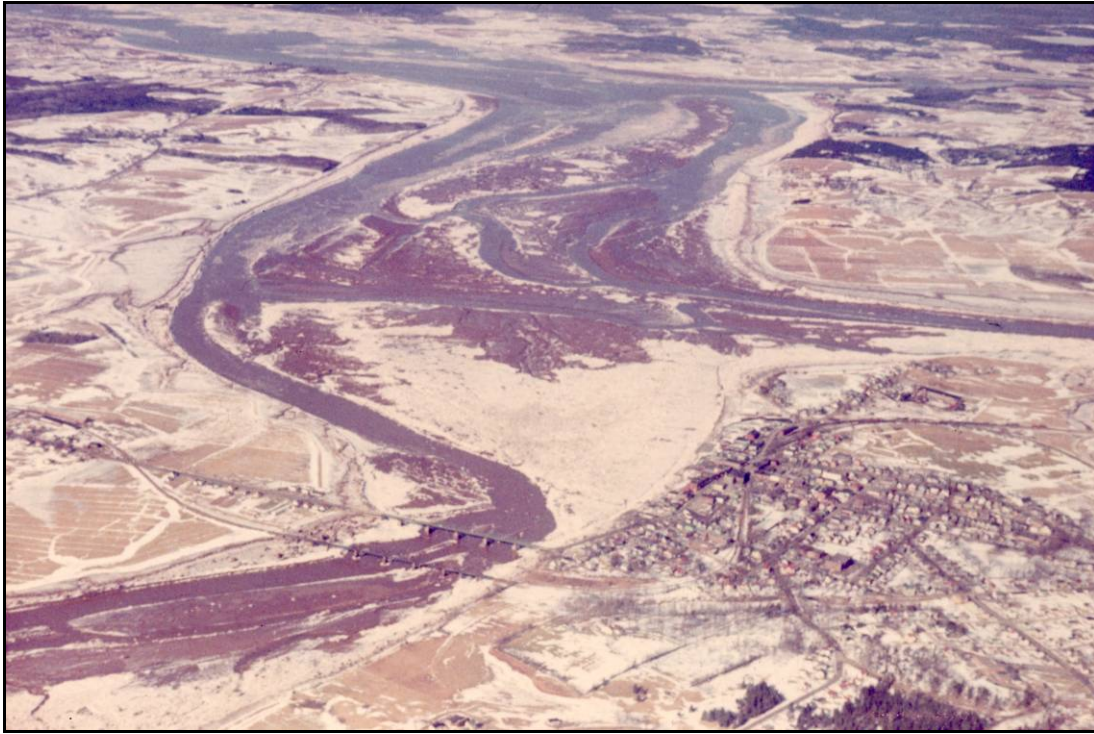
Figure 7: Extensive intertidal flats evident at low tide on the Avon River near the Town of Windsor during the Winter of 1963. This aerial photo demonstrates evidence of natural bar formation in the location of the future causeway. Photo by C.A. Banks, 1963.
