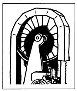
5.10 Feed rolls on resaws shall be guarded when necessary to prevent the hands of the operator from coming in contact with the rolls.
