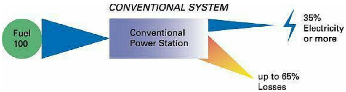
FIGURE 2.5-2 Typical conventional power generation scheme
