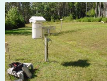
Sherbrooke, Nova Scotia Acid Precipitation Monitoring Station
