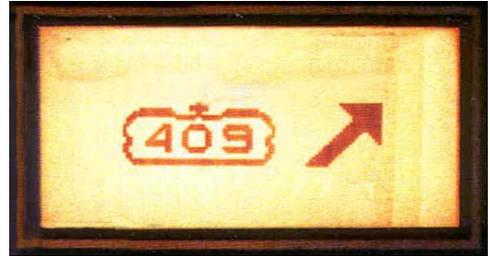
In recent years, there have been extensive amounts of research initiated to increase contrast ratio thus increasing visibility. There are several characteristics that make LCD’s attractive for DMS applications, including completely solid state, compact design, and wide viewing angle. LCD may emerge as a viable DMS technology over the next five years.
