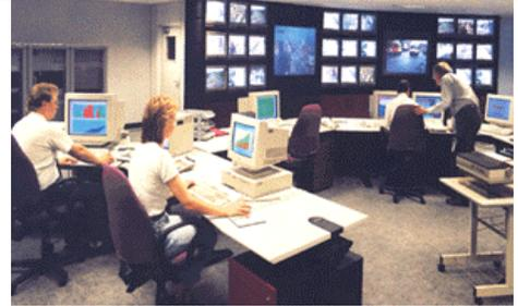
CRT or light valve based rear-projection technology is proven, widely available and provides suitable intensity in office level illumination. The primary drawback for this technology is the space requirements to accommodate the systems.
