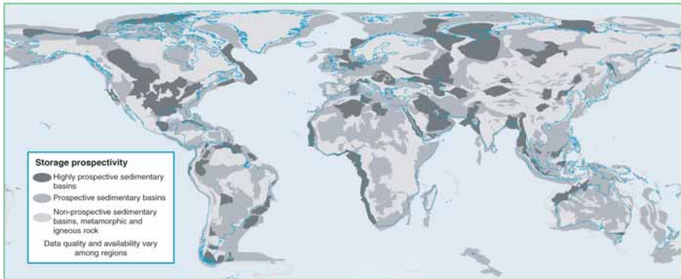
Figure TS.2b. Prospective areas in sedimentary basins where suitable saline formations, oil or gas fields, or coal beds may be found. Locations for storage in coal beds are only partly included. Prospectivity is a qualitative assessment of the likelihood that a suitable storage location is present in a given area based on the available information. This figure should be taken as a guide only, because it is based on partial data, the quality of which may vary from region to region, and which may change over time and with new information (Courtesy of Geoscience Australia).
