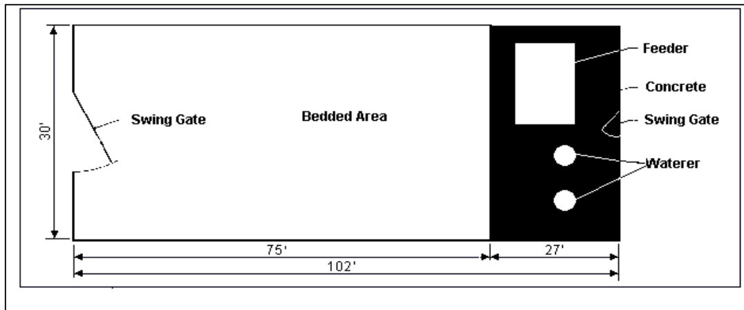
Figure 2 Common layout of a grow finish structure
