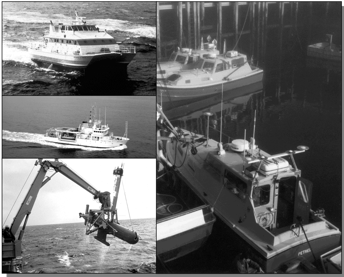
The Canadian Hydrographic Service multibeam sounding platforms: the Frederick G. Creed (upper left); a SWATH (Small Water Area Twin Hull) type vessel; the Matthew (center left); the Dolphin (lower left); and 10-metre-launches (right) fitted with EM3000 sounding systems.
