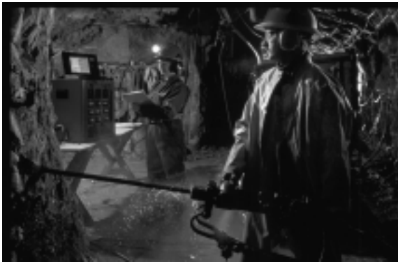
CANDRILL Water-powered rock drill Val-d'Or, Québec
