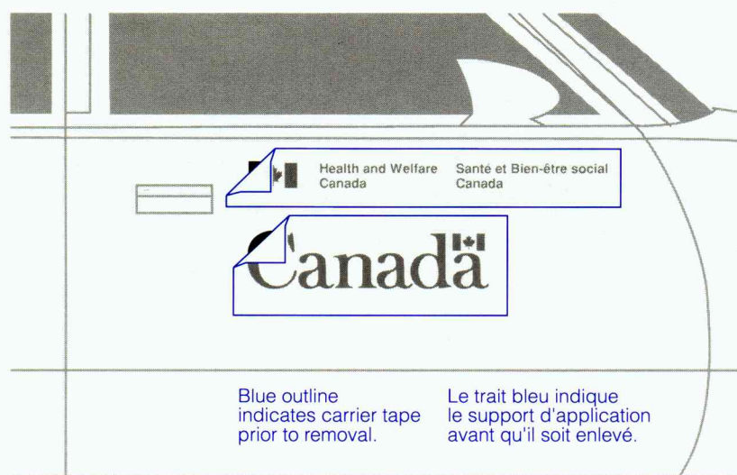
Fig. 11 Installation of decals. Installation des décalques.
