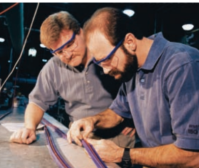
Superior elastomeric material, used in the latest CANDU 6 containment airlocks, is based on technologies that have been used to improve U.S. Space Shuttle performance.
