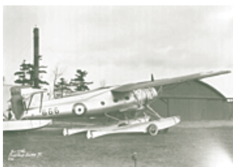
RCAF Fairchild Super 71, Rockcliffe, 1936. This was the first Canadian-built aircraft with an all-metal, monocoque fuselage. (Public Archives of Canada PA 63184)
