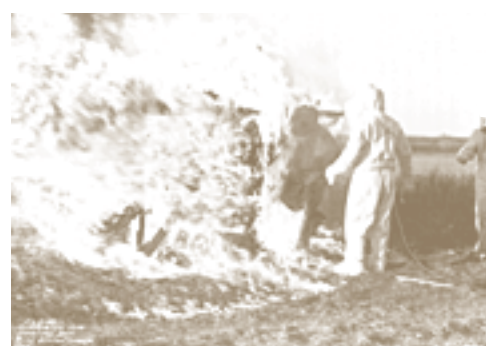
Tests on fog landing equipment and the drop testing of parachutes are examples of the type of investigations that were carried out by the Test Flight in addition to the type testing of new aircraft. Here Mansfield fire-resistant asbestos suits are demonstrated at Rockcliffe in 1939. (Public Archives of Canada PA 63669)
