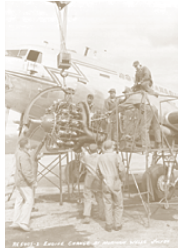
An engine change is being carried out on this Photo Squadron Dakota at Norman Wells, N.W.T., in July 1950. Aircraft heading to their northern bases from Rockcliffe took their own ground crews, including cooks. (Public Archives of Canada PA 66428)
