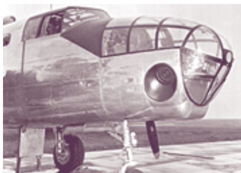
Camera installation on B-25 Mitchell for tri-metrogon mapping process, 1944. (Public Archives of Canada PA 65503)
