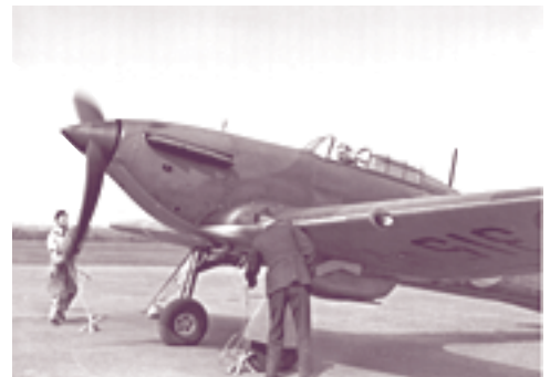
Starting a Hawker Hurricane using a hand crank at Rockcliffe. (Public Archives of Canada PA 63511)
