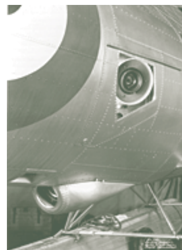
Exterior view of multi-camera installation in a Fairchild Super 71, Rockcliffe, 1936. (Public Archives of Canada PA 63180)
