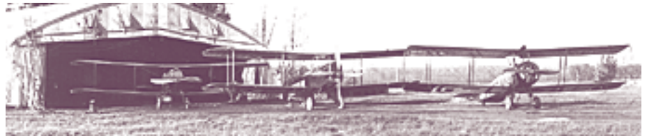
The Bessonneau hangar at Rockcliffe showing a Bristol F.2B in the doorway, with a de Havilland DH-4 and an Avro 504K lined up outside, ca 1922. (Public Archives of Canada PA 62272)
