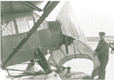
Warming the engine on a Fairchild FC-2 with torch and canvas engine cover in March 1929. (Public Archives of Canada PA 62629)
