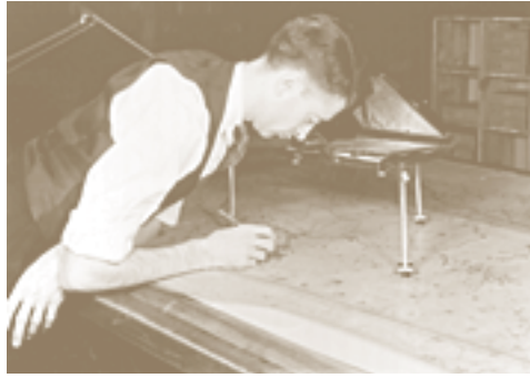
A government technician plots map from information derived from tri-metrogon aerial photographs taken by the RCAF, 1945. (Public Archives of Canada PA 65579)
