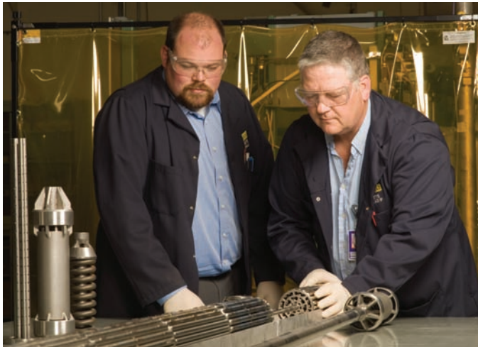
Noel Harrison, Engineering Physicist (left) and Peter Valliant, Metallurgical Engineering Technician, Chalk River. Assembling fuel string.
