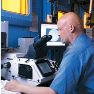
Craig Buchanan, Metallurgical Technician, Chalk River. Optical examination of fuel materials and fuel channel components.
