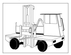
Side Loading Trucks are designed to move long materials by loading them parallel to the direction of travel.
