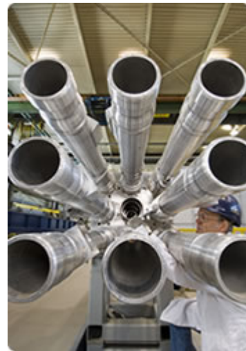
A reactor mock-up is being readied by AECL to play a vital role in extending the life of the Point Lepreau Generating Station.
